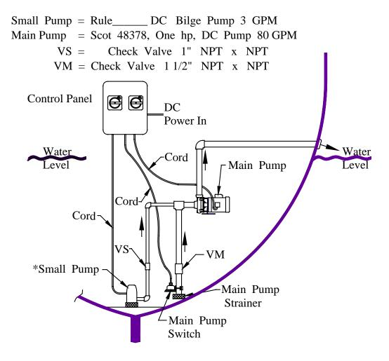
\* Small Pump is usually the vessel's existing bilge pump
